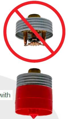
Fully insert the Model W3 wrench over the cap until it reaches the bottom of the cup, or the Model FC wrench over the sprinkler until the wrench engages the body. Do not wrench any other part of the sprinkler/cup assembly. The Model W3 and FC wrenches are designed to be turned with a standard 1/2" square drive. Tighten the sprinkler into the fitting after applying a PTFE based thread sealant to the sprinkler's threads. Recommended installation torque is specified in Table J.
