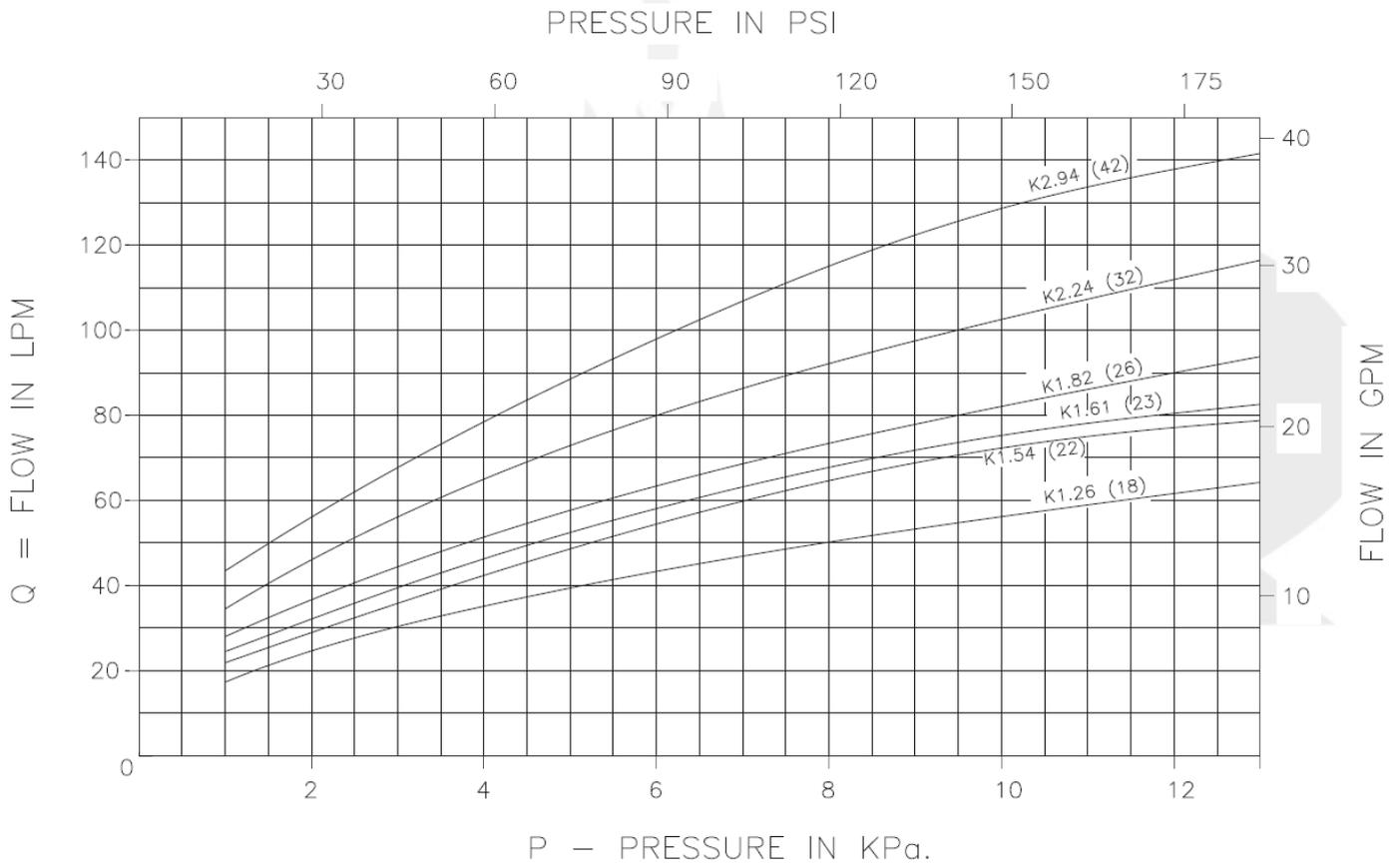
$Q = K\sqrt{P}$ , WHERE P IS SUPPLY PRESSURE IN KPa. & K IS NOZZLE CONSTANT.
