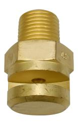
Reliable Models B Open Window, FM Open Window and FM Open Cornice Nozzles are especially designed for external use. They are installed in locations where a blanket of water is desired over a predetermined area. Open Nozzle systems can be operated manually or by quick opening valves that are pneumatically, hydraulically or electrically controlled.
